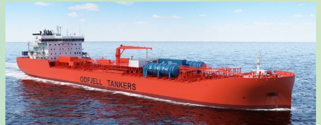
Illustration of the fuel cell installation on board a chemical tanker.
