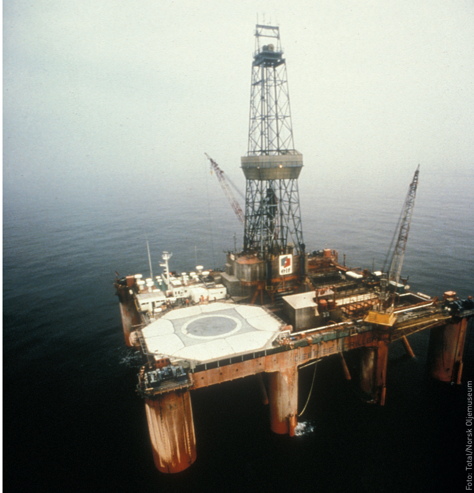
Deep Sea Driller, the very first Aker H3 semi-submersible drilling rig, at the Frigg field in 1975-76. The rig is ordered by Odfjell in 1971 and delivered in 1974. Deep Sea Driller runs aground and capsizes in 1976 while being taken ashore for maintenance, sadly causing the loss of six crew-members.
